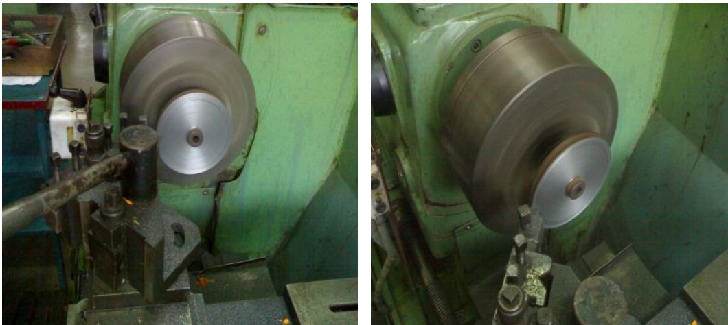
Figure 3.8 Facing of the impeller on machine lathe
