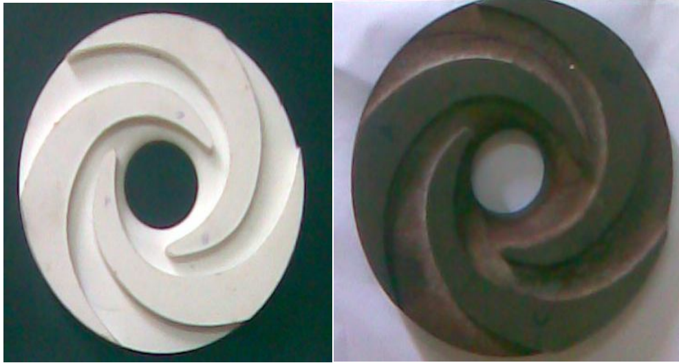
Figure 4.7: Comparison of flow volumes of CI and RPT impeller
